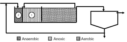
where the denitrification is taking place. The factors affecting the ORP of this zone are also the same as the Bardenpho: the amount of recycled aerobic mixed liquor, the amount of anaerobic effluent from the first zone, along with the biological state of the bacteria from each zone. Like most anoxic zones, the ORP should be between -100 and 100 mV.
