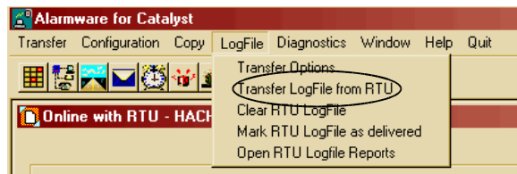
Figure 76: Transfer LogFile from RTU
